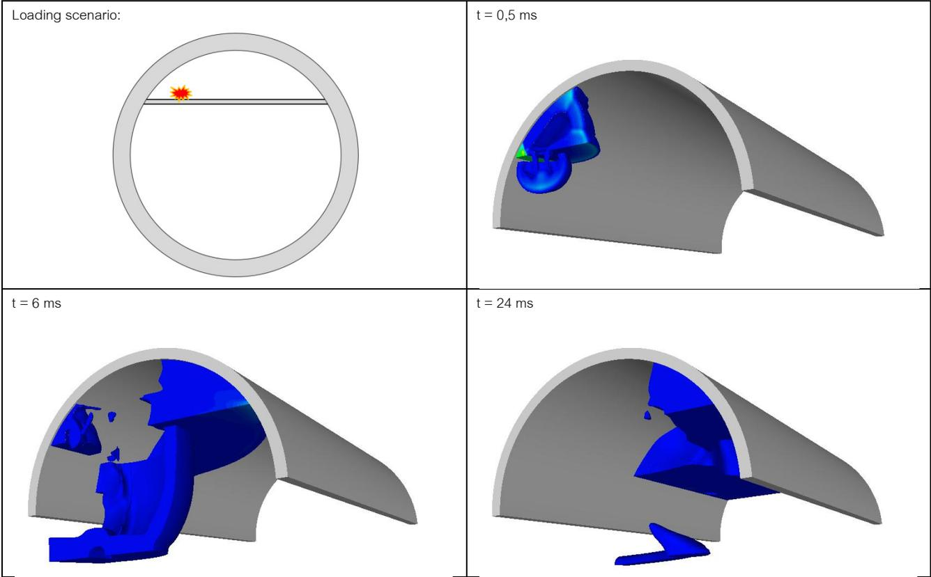
Figure 2: Propagation of the shock wave resulting from a detonation at the intermediate slab of a tunnel
